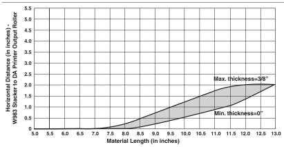
The top chart is used to determine the distance to set between the Stacker deck and the DA Printer output roller. This is done by adjusting the height of the stand. The bottom chart is used to determine the distance from the Stacker to the output roller. This is done by moving the Stacker closer or farther from the DA Printer output roller. In order to use the charts:
